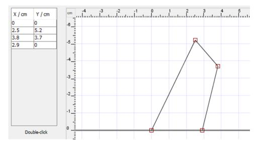
We have used the original fins provided in the kit. These fins had a tapered swept shape. Fin shape and dimensions:
